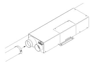
**Important:-** Ensure that a minimum of one hot air outlet vent is permanently open at all times. This should ideally be the first outlet and not more than approximately 1 metre from the heater.
