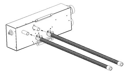
Push on the ends of the flues with the blue adaptor to the pipes on the underside of the Space Heater ensuring they are fully pushed on, and secure with supplied hose clips.
