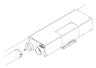
**Important:-** Ensure that a minimum of one hot air outlet vent is permanently open at all times. This should ideally be the first outlet and not more than approximately 1 metre from the heater.
