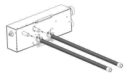
Push on the ends of the flues with the blue adaptor to the pipes on the underside of the Space Heater ensuring they are fully pushed on, and secure with supplied hose clips.
